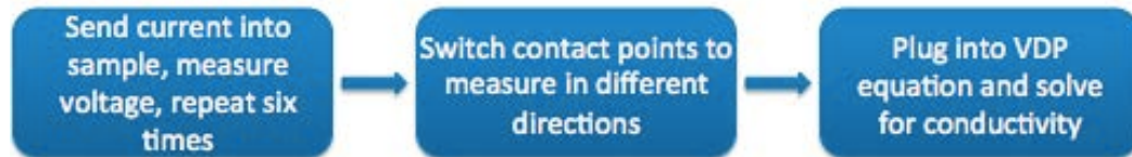
Figure 24. High-level overview of measurement setup for Van Der Pauw method
