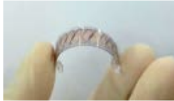
Figure 11. TEG screen printed onto a glass fabric [22]
