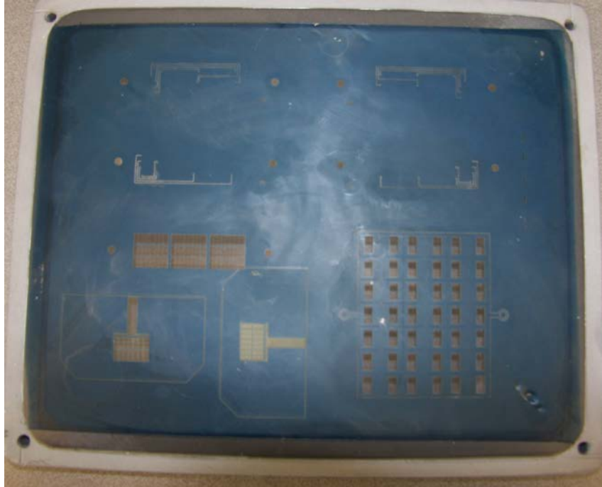
Figure 18. Processed screen with patterns rastered out for screen-printing
