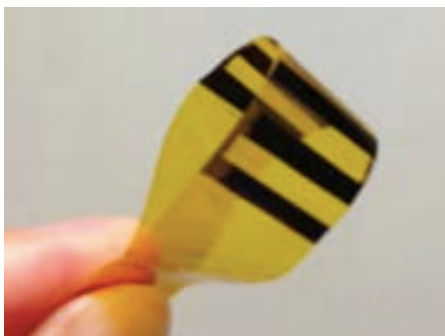
Figure 9. Ink-jet printed thermoelectric device on Kapton [54]
