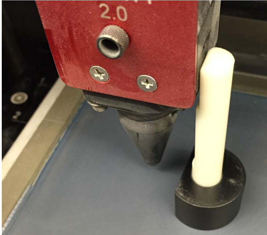
Figure 17. Tool used to align height of laser to surface of screen
