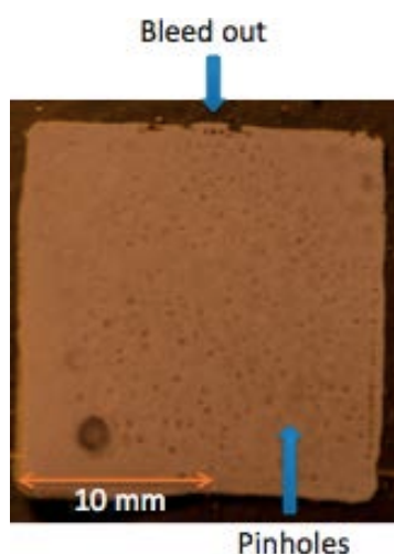
Figure 23. Example of bleed out and pinholes occurring in a print
